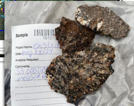
A sample of uranium mineralization hosted within massive biotite pegmatite discovered on the Eastside property.
