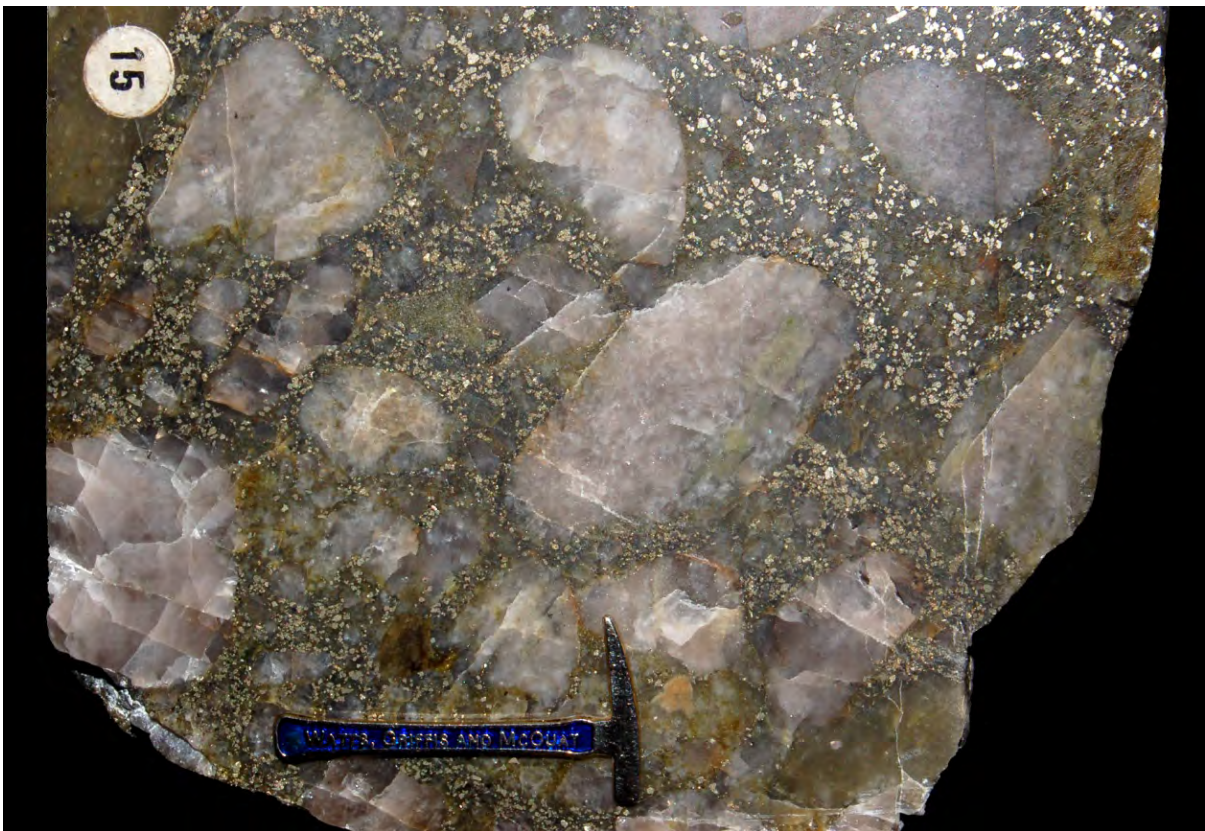
Plate 2: Typical Elliot Lake ore from the Matinenda Formation – compact, well indurated quartz-pebble conglomerate with detrital pyrite and interstitial uranium minerals – 3 cm hammer scale.
