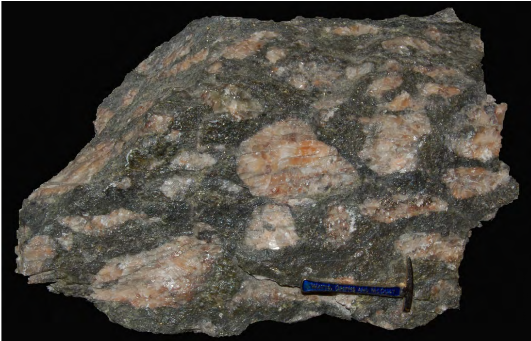
Plate 4: Elliot Lake ore - rounded quartz pebbles in U-bearing, sulphide-rich matrix – 3 cm hammer scale.
