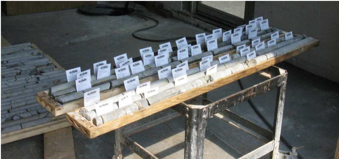
Plate 10: Two core trays with sample tags inserted at selected intervals prior to cutting.
