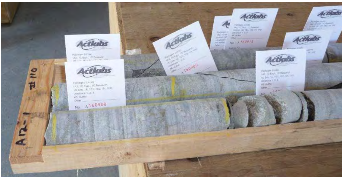
Plate 11: Close-up of core tray with sample tags inserted at selected intervals and cutting line marked prior to cutting.
