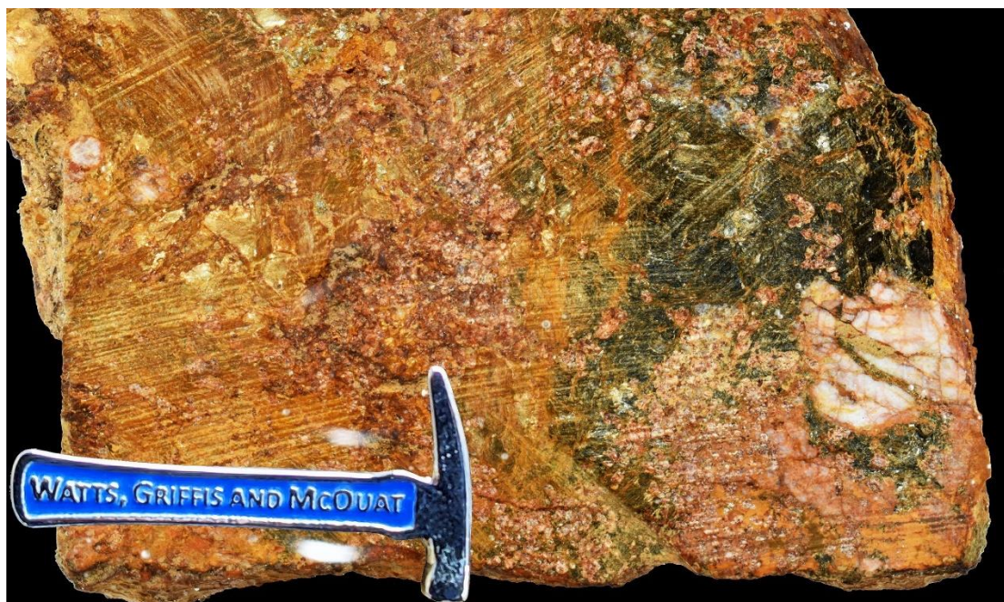
Plate 1: Photo of brecciated Fe-stained pegmatite on SE-trending shear in the Wilson Zone
