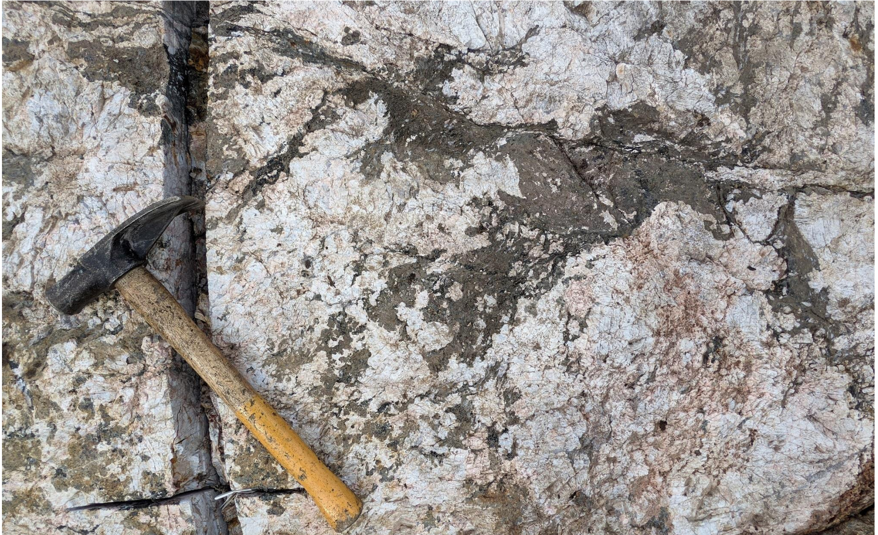
Plate 14: Detailed photo of the central part of Plate 11 showing dark green biotite-monazite mineralization filling voids in pegmatite as a result of brittle-ductile shearing. This location produced 15,000 to 18,000 cps (total count).
